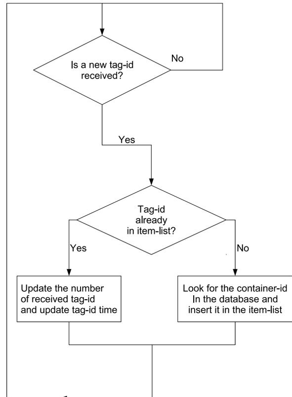
Fig. 1. Flowchart for processing the received tag identifiers.
