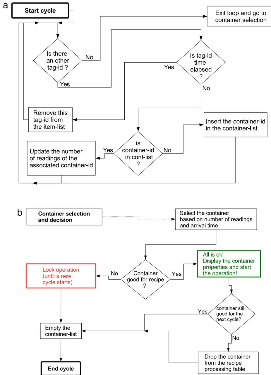
Fig. 2. Tag list processing (a) and container selection (b) flowcharts.
