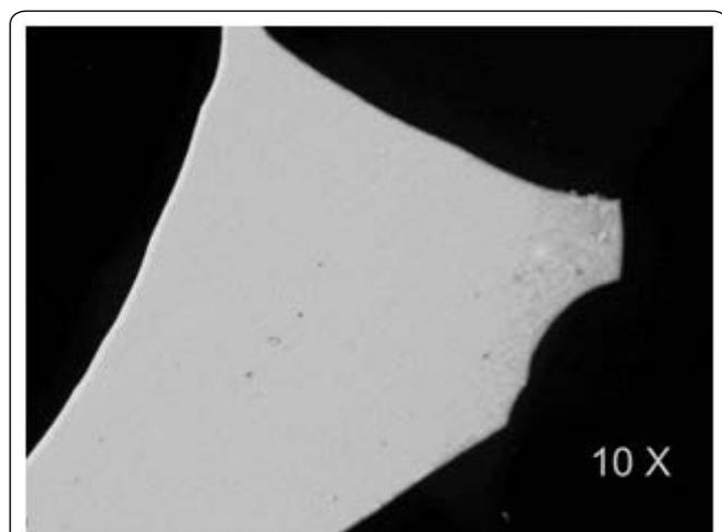
Figure 1: Anodic porous alumina fragment 10X magnification.
