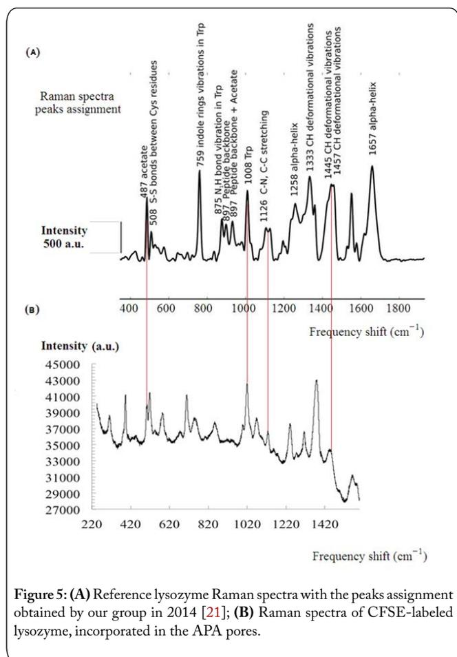
**Figure 5:** (A) Reference lysozyme Raman spectra with the peaks assignment obtained by our group in 2014 [21]; (B) Raman spectra of CFSE-labeled lysozyme, incorporated in the APA pores.
