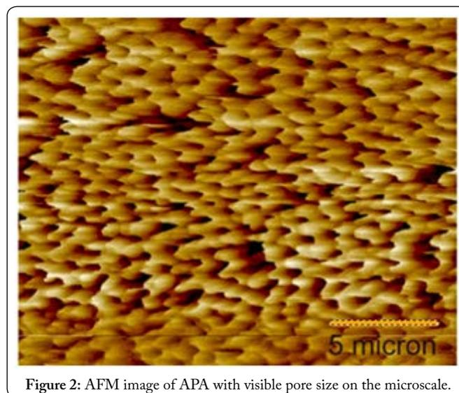
Figure 2: AFM image of APA with visible pore size on the microscale.
