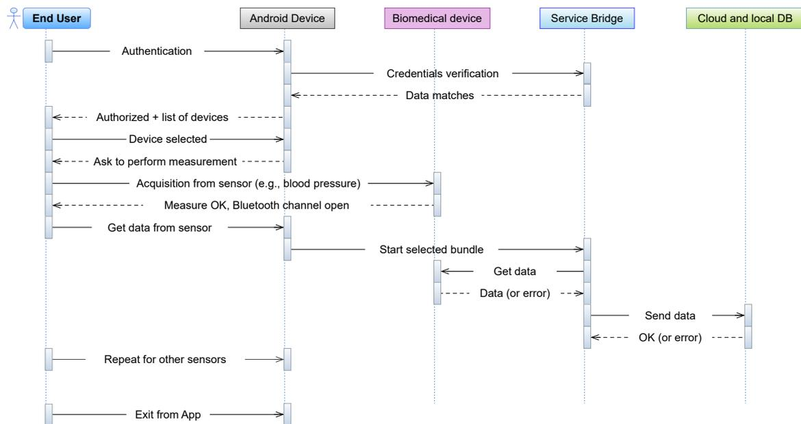
**Figure 7.** Overview of how the user interacts with the *Health App* and performs a measurement.
