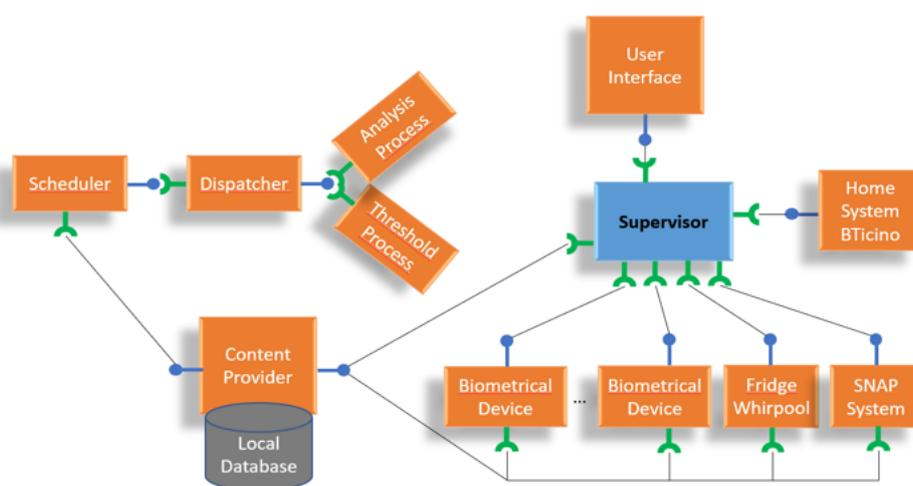
Figure 5. The developed bundles architecture.
