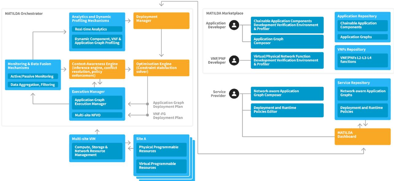
Figure 2. MATILDA 5G High Level Architectural Approach.
