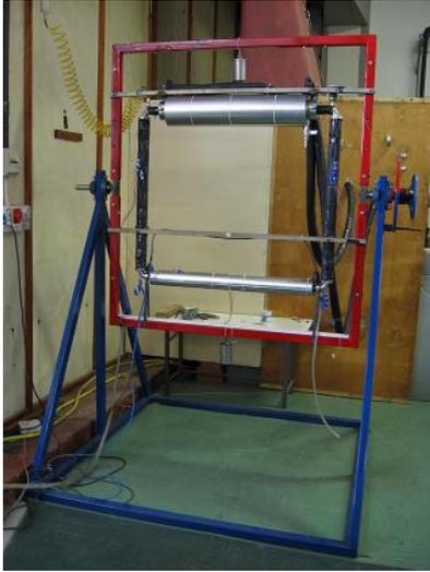
**Figure 1.** Experimental natural circulation loop [9]
