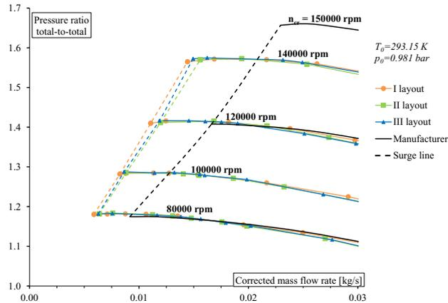
Fig. 6. View of surge margin for each layout considered and in the case of turbocharger manufacturer.
