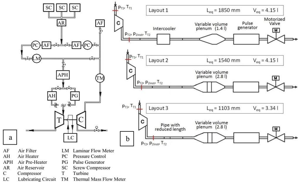
Fig. 1. Schematic layout of University of Genoa test facility (a) and downstream compressor circuit layouts (b).
