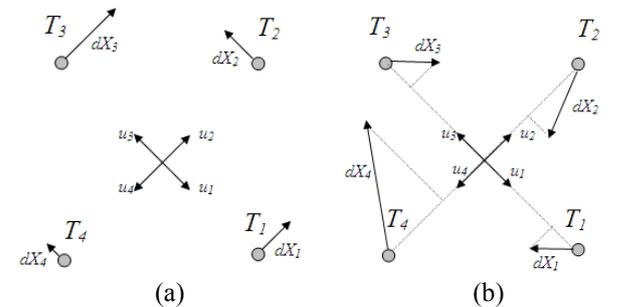
Fig. 4 – Scenarios of null contribution provided by  $b_i$  terms. a) every  $b_i$  term is null, as every  $dX_i$  vector is orthogonal to its corresponding  $u_i$ ; b)  $b_i$  terms are not null but their resulting contribution to error vector  $e$  is null
