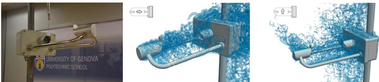
**Figure 2:** Image of the Thies LPM optical NCG installed in the DICCA wind tunnel (left-hand panel). Visualization of the turbulent structures around the gauge body using the Q-criterion on the LES results for a wind direction of  $\alpha = 0^\circ$  (central panel) and  $\alpha = 90^\circ$  (right-hand panel), at a wind speed of 5  $\text{m s}^{-1}$
