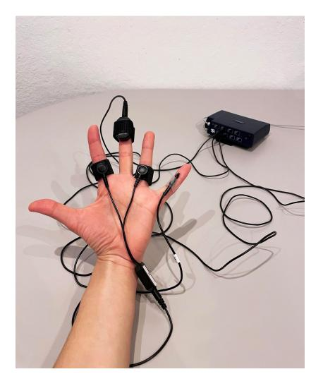
**30** The *skin temperature* (ST) sensor is designed for continuous temperature monitoring using the skin as an indicator of body temperature, rising in response to higher levels of arousal, independent of valence.
