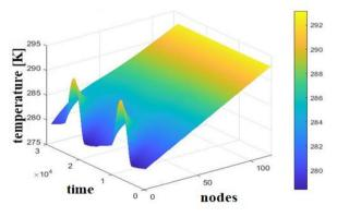
Figure 5. Thermal distribution in MLP03 with polyurethane foam as insulator in January.
