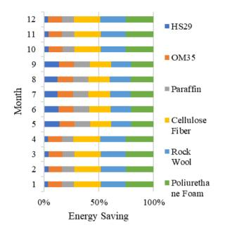
Figure 2. Energy saving for standard insulators or PCMs compared with MLP03 wall.
