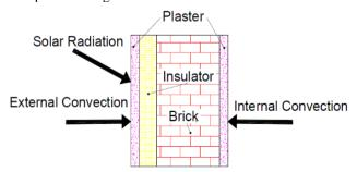
Figure 1. Schematic of the configuration under investigation.
