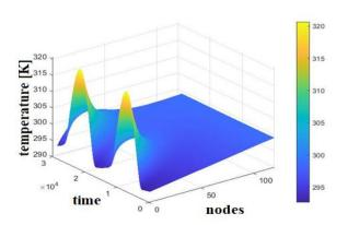
Figure 6. Thermal distribution in MLP03 with polyurethane foam as insulator in July.
