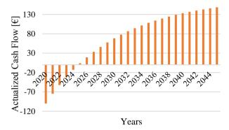
Figure 7. Actualized cash flow for rock wool, in MLP03 conditioned by heat pump alone. Payback is guaranteed in 2025.
