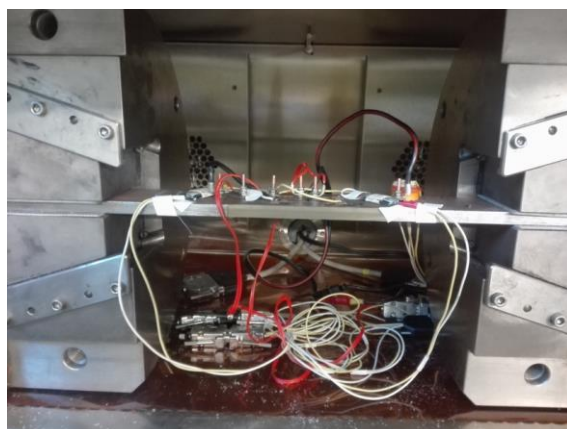
Figure 21: Middle tension specimen equipped for crack growth rate measurement by direct current potential drop method with crack detection gauges and PT100 resistance thermometers
