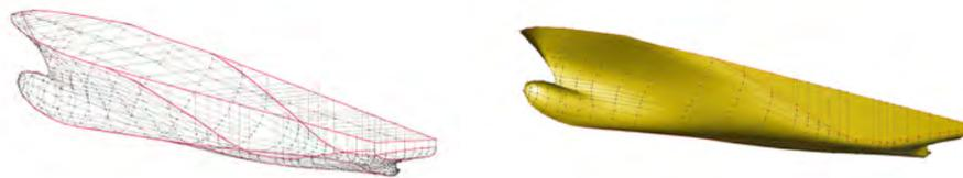
**Figure 6.** Example of the initial DTC test case geometry: the control net (**left**) and the smooth surface (**right**).
