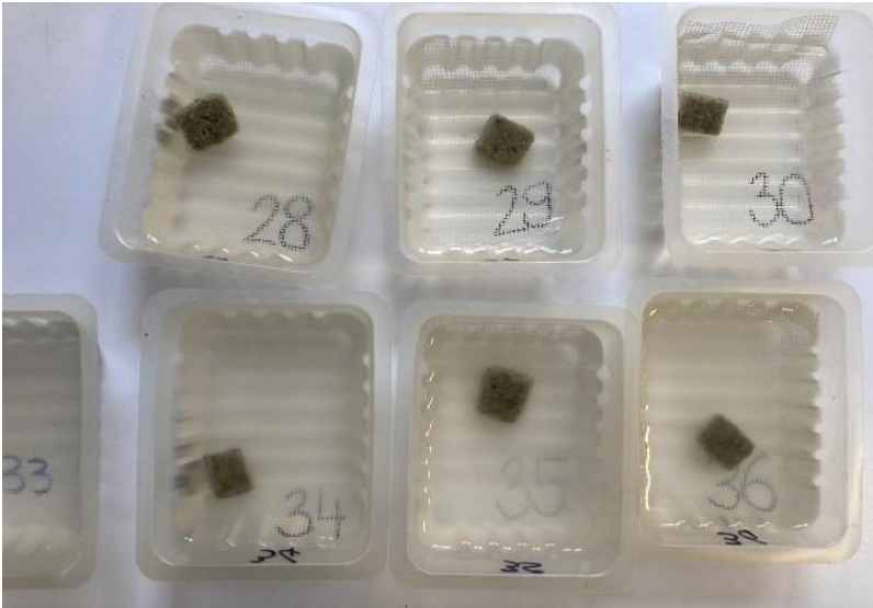
Figure 5.4: status of the feed after 48h in seawater for the new formulation.
