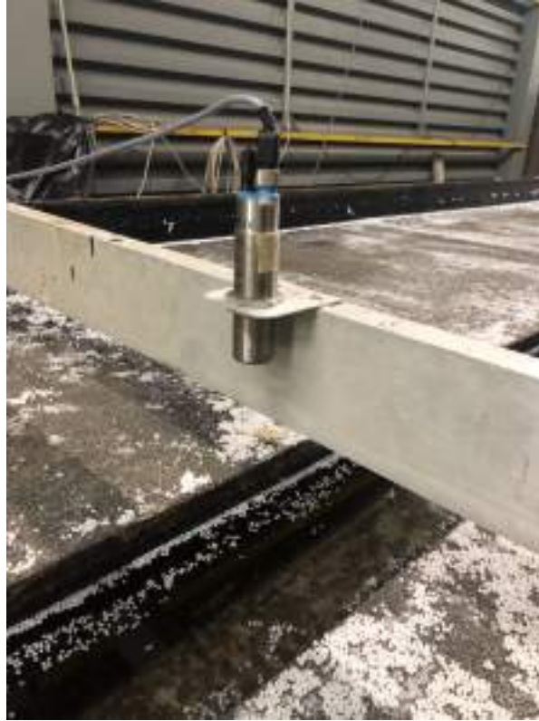
Figure 2.3: Ultrasound Gauge detail.
