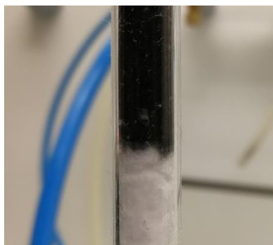
Fig. 3 – Char (above) and quartz wool (below) inside the quartz-tube reactor.
