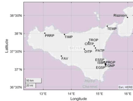
Fig. 4. Locations of the synchronous machines in the Sicilian network. The slack generator is located on the peninsula in the substation of Rizziconi.
