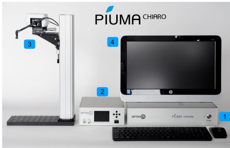
Figure 9 CHIARO indenter main elements (1) the controller, (2) the interferometer, (3) the head, (4) the pc.
