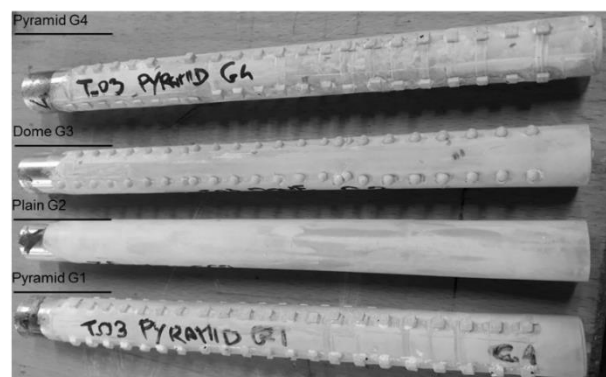
Figure 7. Exhumed model piles some with profiled bores
