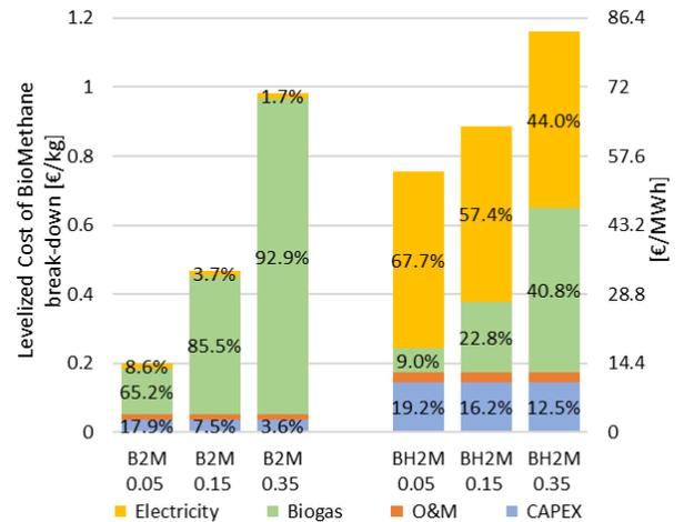
**Fig. 4.** LCOBM for the proposed plants at different biogas costs (0.05-0.15-0.35 €/m<sup>3</sup>)
