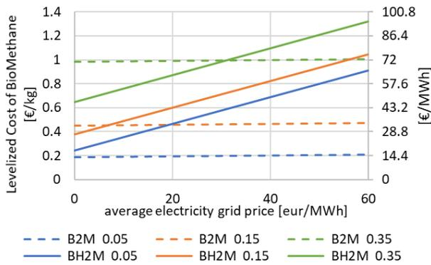
**Fig. 6.** Levelized cost of biomethane as function of the average grid electricity price; parameter biogas cost (0.05-0.15-0.35 €/m<sup>3</sup>)
