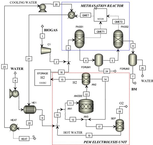
Fig. 3. Flowsheet of the BH2M plant model
