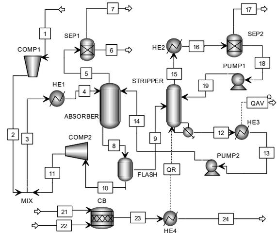
Fig. 2. Flowsheet of the B2M plant model
