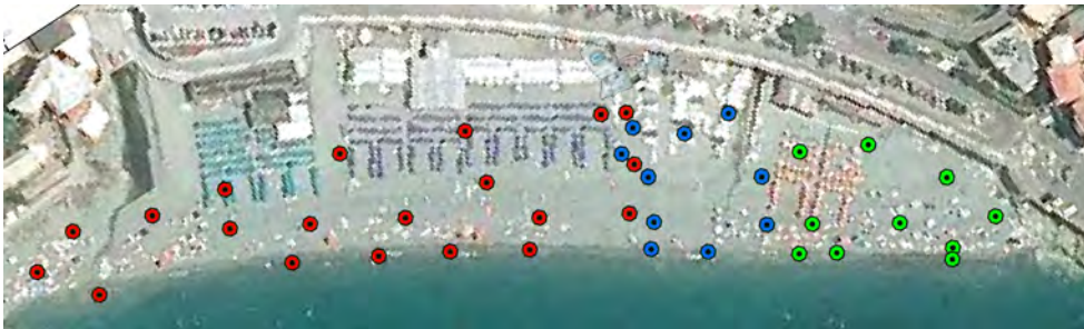
Figure 6: GCPs acquired for each Camera: western (red points), central (blue points), eastern camera (green points)
