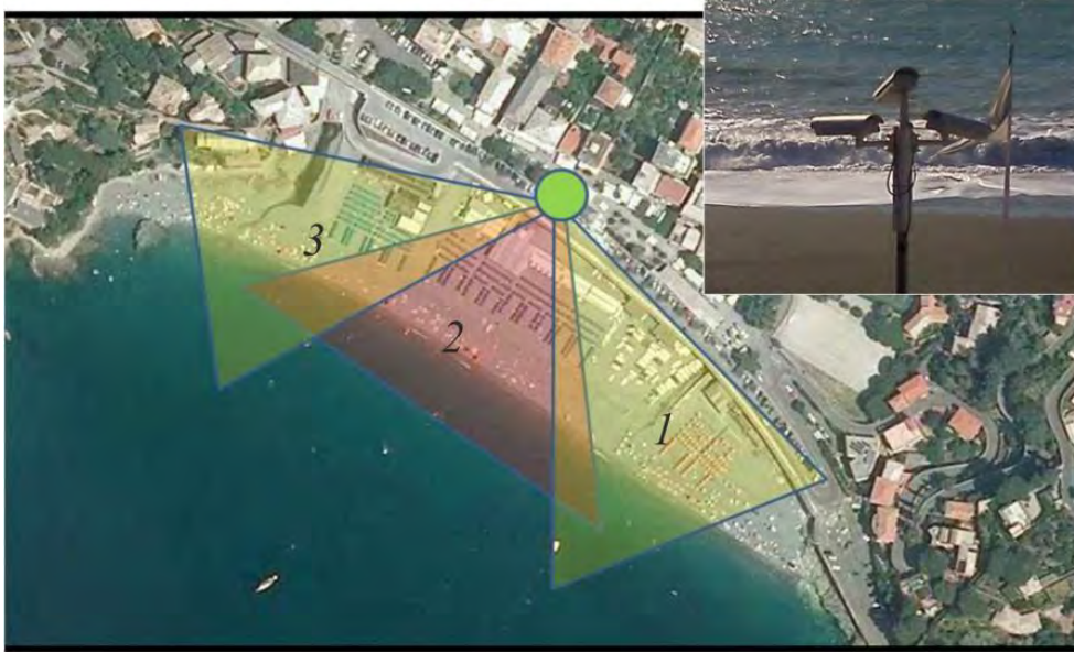
Figure 5: Bonassola camera system configuration
