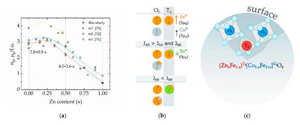
**Figure 3.** (a) Dependence of net magnetic moment per formula unit for cobalt ferrite nanoparticles doped with zinc from this research compared with reference systems [25,32,51]; (b) diagram of the evolution of the magnetic structure of cobalt ferrite when is doped with zinc; (c) illustration of spinel structure of co-doped Zn-Co ferrite: in nanoferrites the octahedral  $(O_h)$  positions of spinel preferably allocated on the surface rather than tetrahedral  $(T_d)$  positions.
