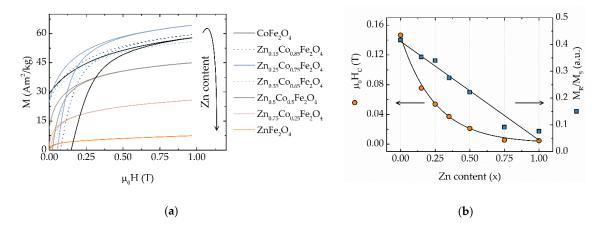
**Figure 2.** (a) The first quarter of M-H hysteresis cycles recorded at 300 K of  $CoFe_2O_4$  nanoparticles doped with Zn. The arrow indicates the trend of  $M_S$ ; (b) Dependence of coercivity  $H_C$  and reduced remanence  $M_R/M_S$  versus Zn-content.
