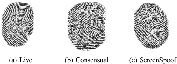
Fig. 5: Example of live and spoof images adopted in the test stage of the LivDet 2019 algorithms.
