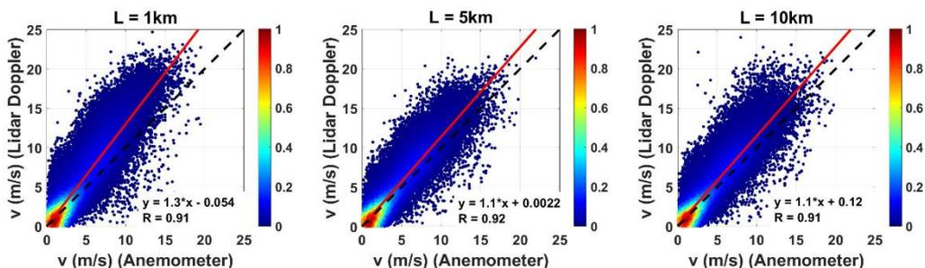
**Figure 1.** Wind speed retrieved by SingleDop using the Doppler lidar scans at 2.5° as a function of the anemometer measurements. Three de-correlation lengths ( $L$ ) are shown: 1 km, 5 km and 10 km. The colour of points represents the relative density of points.
