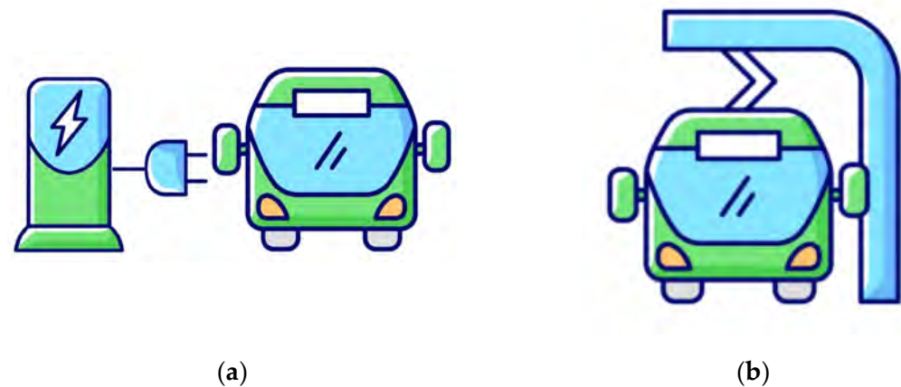
Figure 14. Representation of (a) depot and (b) opportunity charging systems.
