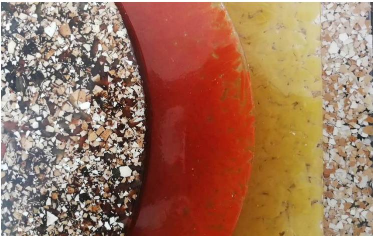
Figure 3. Bioplastic combination with eggshell, pasta, lentils. Bis Bioresina G. Centineo, M. Lequio, Li Changrui, Shi Xinran. Ph. M. Paolillo
