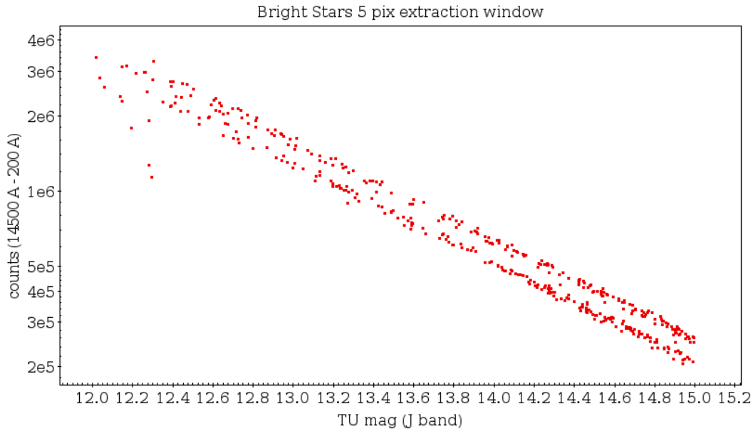
Figure 3.8: Flux-magnitude relation for extracted spectra in a simulation with only bright stars and no background. The flux on the y axis is measured in photon counts. Two different linear trends are clearly visible in the counts-magnitude relation. Plot courtesy of Marco Scodreggio.
