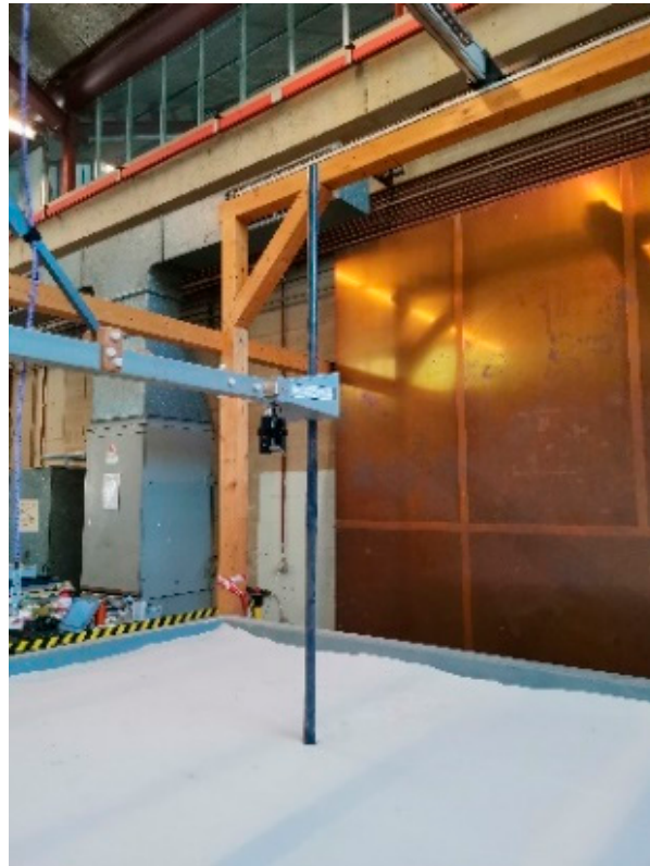
Figure 3. Detecting the cylindrical model with the lightweight radar system with vertical polarization.
