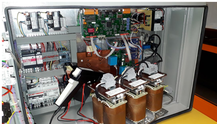
Fig. 16. Experimental setup: Three-phase inverter, modified according to the schematic shown in Fig. 15; Two inductances only have been actually used.
