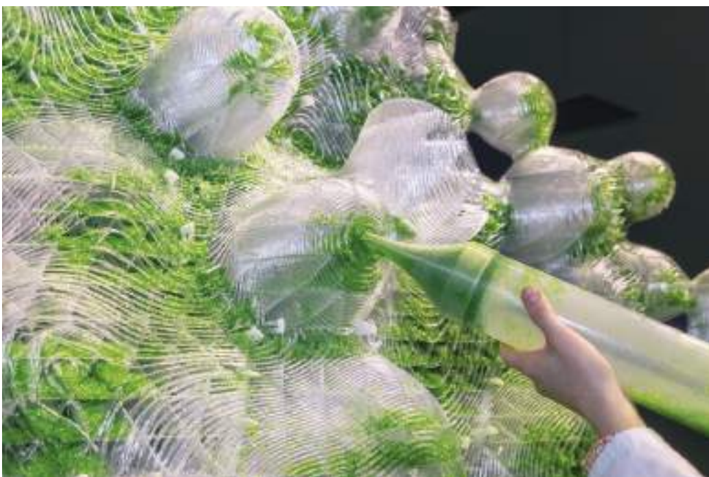
Fig. 11-13 | H.O.R.T.U.S. XL Astaxanthin.g. The world's first 3D-printed bioreactor. The installation, on display at the Centre Pompidou of Paris for the La Fabrique du Vivant exhibit, is understood as a 1:1 prototype of living architecture – a new generation of biophilic architectural skin inserted into urban life. The structure is algorithmically designed and produced through high-resolution, large-scale 3D printing. Among the oldest organisms on Earth, the exclusive biological intelligence of cyanobacteria is collected as part of a new form of bio-digital architecture. Design: ecoLogicStudio (C. Pasquero, M. Poletto, K. Alexopoulos, M. Baldissarra, M. Brewster); Research Partner for biological as well as 3d printed systems and production development: Synthetic Landscape Lab, IOUD, Innsbruck University (Prof. C. Pasquero, M. Kuptsova, T. Greskova, E. Rando, J. Burkart, N. Jabadari, S. Posch), Photosynthetica consortium; Research Partner for 3d printed systems and production development: CREATE Group/WASP Hub Denmark – University of Southern Denmark (Prof. R. Naboni, F. Magaraggia); Engineering: YIP Structural Engineering, M. van de Worp; Microalgal Medium Material Support: Ecoduna AG; 3D printing Material Support: Extrudr (photos by NAARO).
