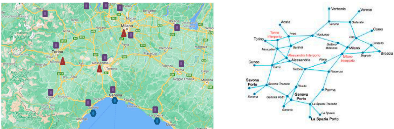
Figure 3. The transportation network of the area under study and the related graph model.
