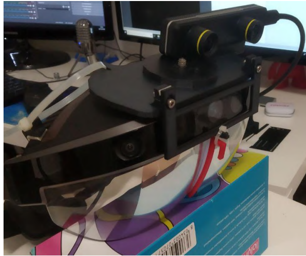
Figure 9: Calibration of the ZED camera with the Meta2 camera to obtain the transformation matrix {}^Z_C\mathbf{T} .
