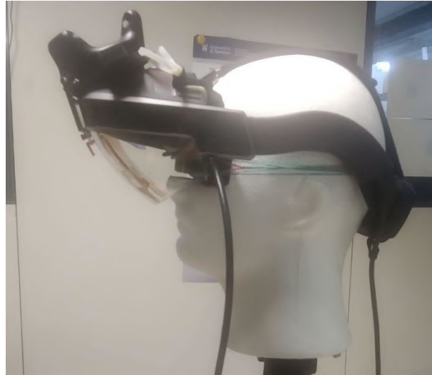
Figure 11: The mannequin head used to validate the HMD registration.
