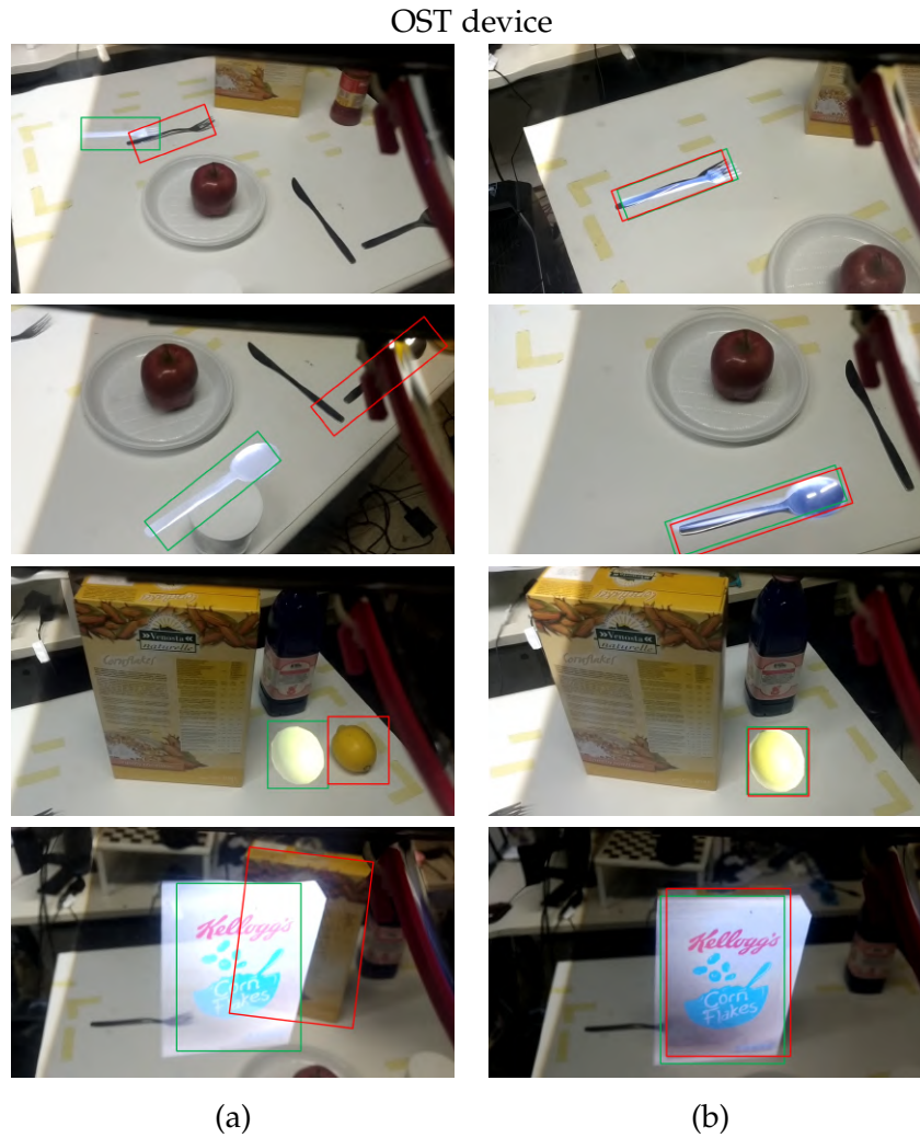
Figure 28: The same representation displayed in Figure 27, but for the OST HMD: before, column (a), and after the alignment, column (b).
