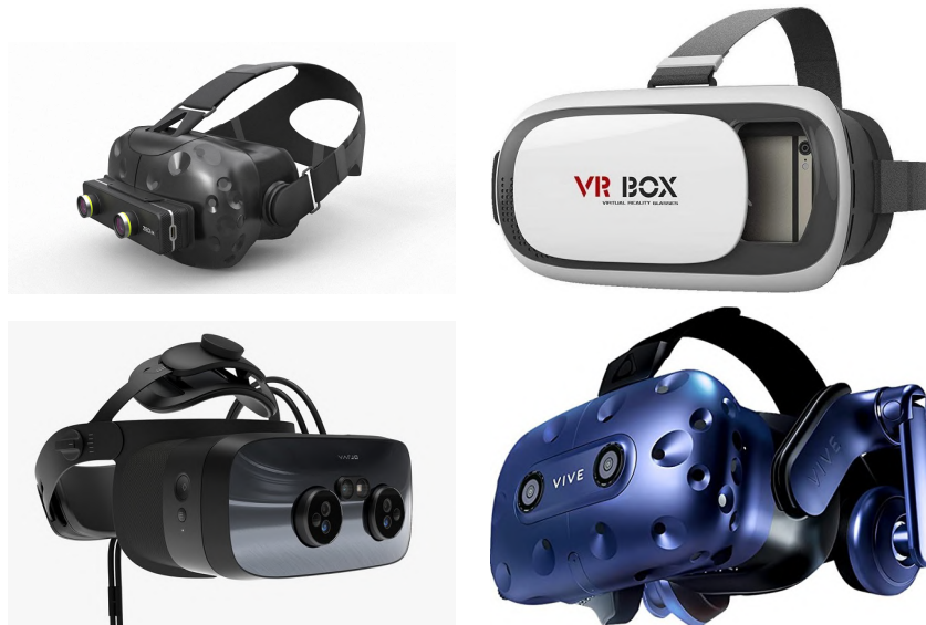
Figure 4: Some examples of commercially available VST HMDs: ZED mini with HTC Vive/Oculus Rift (top left), Google Cardboard (top right), Varjo XR-3 (bottom left), Vive Pro (bottom right).
