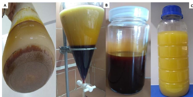
Figure 2. Illustration of the process for obtaining the biosurfactant from Starmerella bombicola ATCC 22214: (A) culture medium containing the biosurfactant produced and isolated in a separating funnel; (B) isolated biosurfactant, and (C) commercial biosurfactant formulation.
