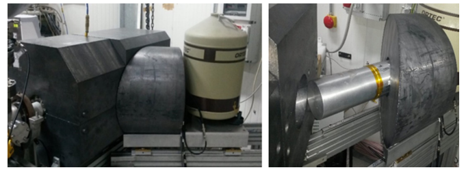
FIG. 2. Lead shielding in the HPGe configuration. Left: close detector geometry (closed shielding); right: larger detector distance (open shielding).
