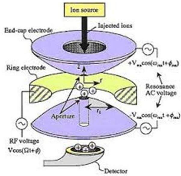
**Fig. 5** Ion trap analyser. The separation takes place within the space between the electrode "covers" and the ring electrode.
