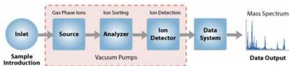
Fig. 2 Block diagram of a mass spectrometer, modified from premierbiosoft.com.
