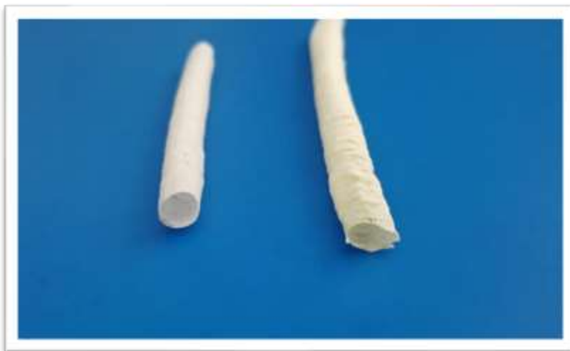
Figure 27. representative scaffold made of PCL:PGS (1:1) (left) and one functionalized with Q (right).
