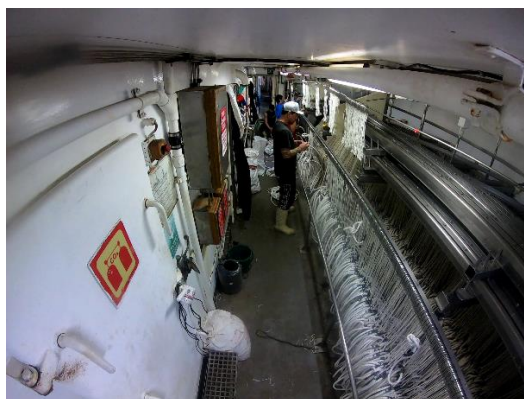
Fig 12. Preparation of the longline before the baiting and the deployment. The system automatically brings the longline there after the hauling and move it for the baiting and deployment, the fishermen just change lost or damaged hooks.
