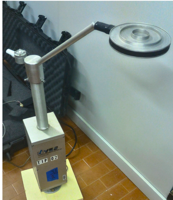
FIG. 1. The hotplate precipitation gauge and a close view of the measuring plate.
