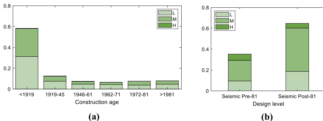
Fig. 3 Class distribution for M a and RC b buildings from the post-earthquake dataset
