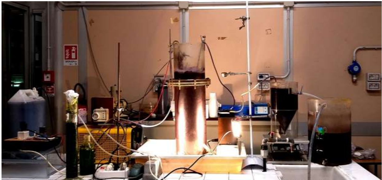
Figure 3.1 The schematic of the lab-scale MPBR configuration and WWW treatment process. 1,9- collection tank; 2,8- peristaltic pump; 3-volume controller; 4- tubular photobioreactor; 5- membrane; 6- pH controller; 7- air pump.
