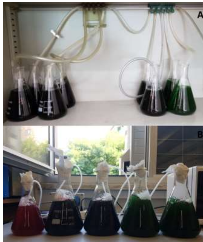
Figure 2.7. Erlenmeyer flask for co-culture growth and winery wastewater treatment: A-under dark conditions, B-under light-dark cycle.
