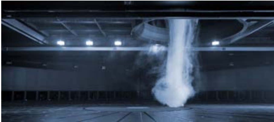
FIGURE 1.13: Simulation of a downdraft in the WindEEE Dome, at the University of Western Ontario; source: www.navigator.innovation.ca .
