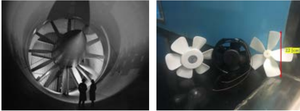
(A) Altitude Wind Tunnel (AWT) Fan, 1944; (B) Three models of the prototype fan, for a multiple-fan wind tunnel. source: www.nasa.gov .
