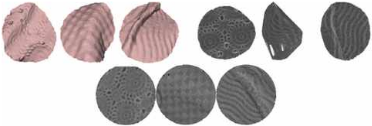
Figure 1.5: Images obtained mapping the mean curvature evaluated on patch vertices onto the parametrization coordinates. Top row, left: mesh renderings. Top row, right: images obtained with the best fitting plane. Bottom row: images obtained on boundary constrained parametrization (after geodesic circle cropping). Image from [Gia18].
