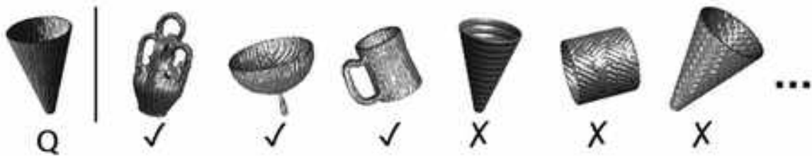
Figure 2: A visual representation of the pattern retrieval problem. A query model Q with a bark-like pattern impressed on its surface is selected. In the ideal case, models with bark-like patterns are retrieved before then models with different reliefs, independently of the global geometry of the models. The "check" and "cross" marks highlight models that are relevant or non-relevant to the query.
