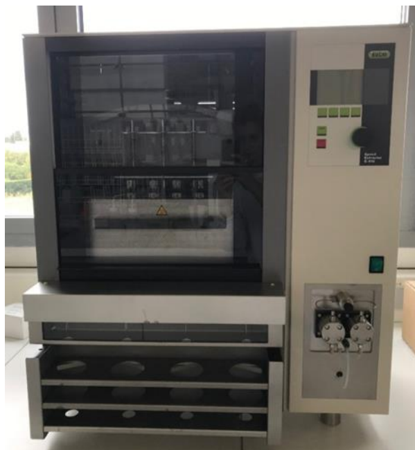
Figure 6. SpeedExtractor (E-916/E-914, BUTCHI, Switzerland) employed for Accelerated Solvent Extraction. University of Avignon, France.
