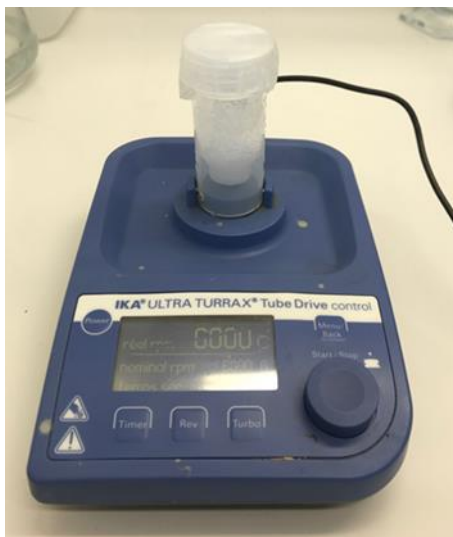
Figure 5. ULTRA-TURRAX® Tube Drive (UTTD, Ika, Germany) employed for Bead Milling Extraction. University of Avignon, France.
