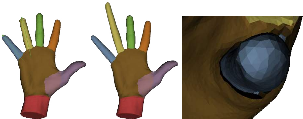
Figure 5.19: The issue related to the “Proportion” constraint. On the left, the original shape with the measures highlighted. In the middle, the ring finger is stretched and the little finger follows. On the right, a zoomed-in view from above of the little finger (the darker part is the interior of the hand).
