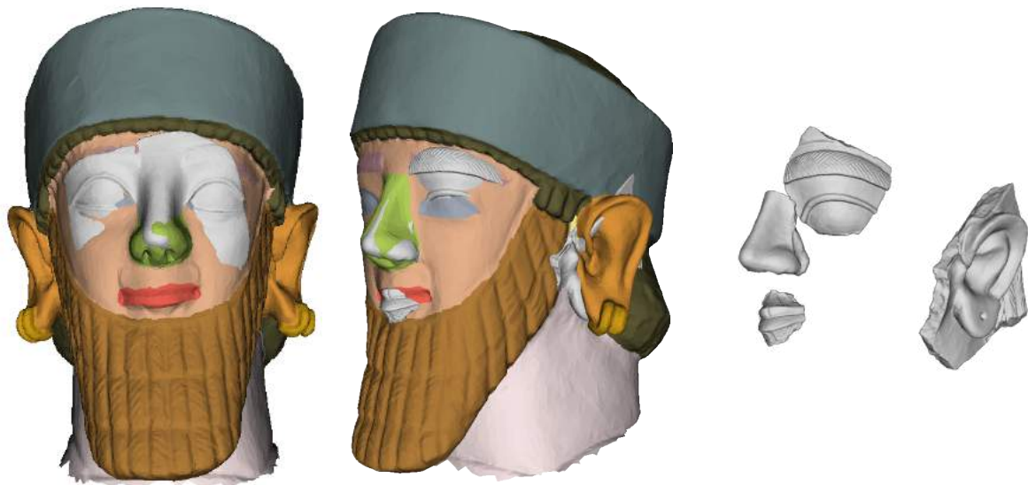
Figure 5.14: The results of the rough alignment obtained employing Umeyama's algorithm.
