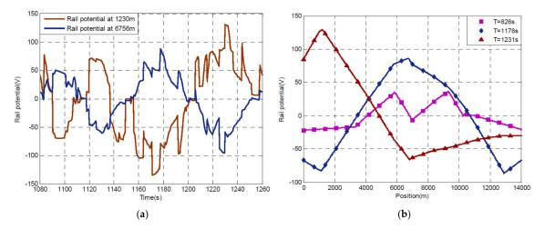
**Figure 5.** Example of track voltage variability vs. time (**a**) and position along the track (**b**). Reproduced from [7].
