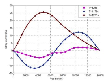
Figure 6. Example of stray current vs. position along the track. Reproduced from [7].
