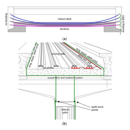
**Figure 1.** Details of (**a**) a viaduct span with tendons (earthed at one end only), (**b**) a viaduct deck and pylon with sketch of the earthing system (in dark green) and of the stray current protection system (SCPS) (in red for stray current drainage (SCD) elements, in brown for the bonding connection and stray current collector (SCC)).
