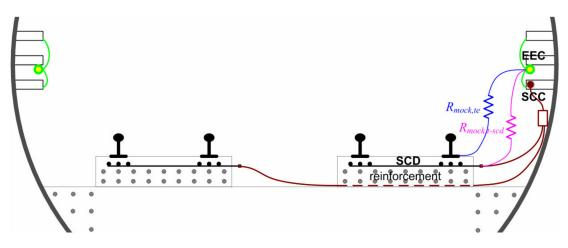
**Figure 8.** Arrangement of artificial leakage test for track alone (in blue) and track and SCD (in blue and magenta), simulating current values in line with pre-existing proportionality and the estimated SCP efficiency.
