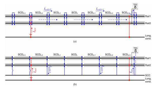
**Figure 4.** Typical SCPS arrangements and measurement of SCP efficiency: (**a**) SCPS without SCC and daisy-chained SCDs; (**b**) SCPS with SCC and isolated SCDs. SCPS elements are in blue; the test circuit is in red.
