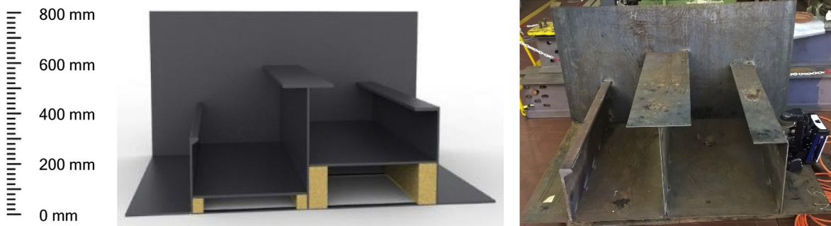
Fig. 9. Obstacle Crossing. Crawlers should cross the beams to inspect selected points of the structure, by simulating different situations changing the height of the obstacles.
