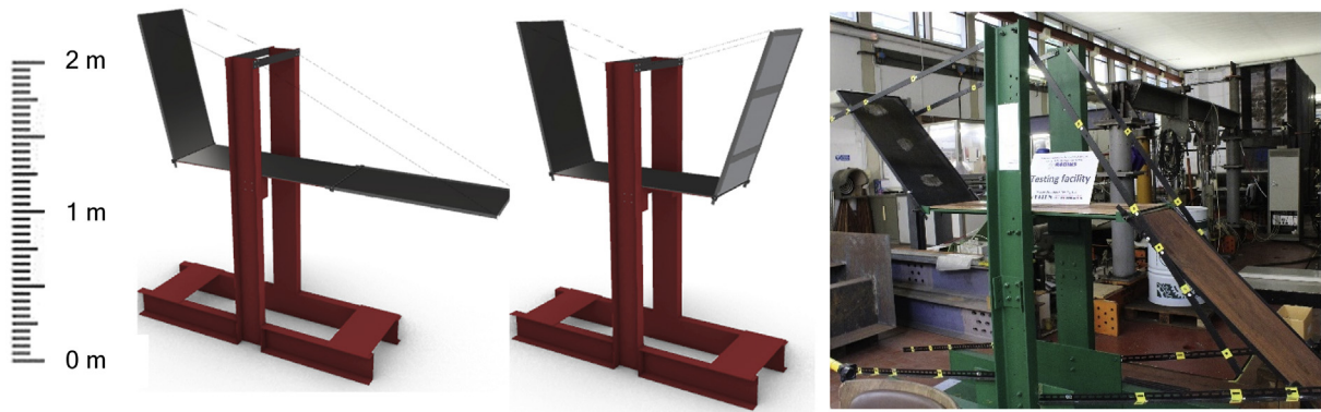
Fig. 10. Adhesion Test. Crawlers should stand still without slipping or moving on tilted surfaces with deposits, measuring the thickness of the plates at each step.
