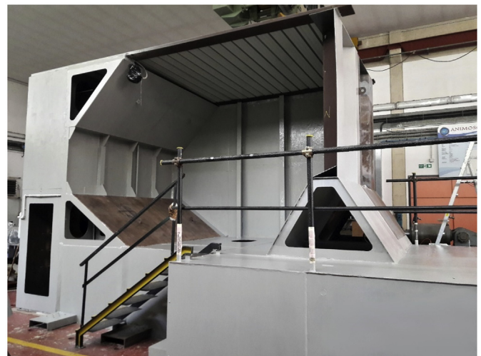
Fig. 4. Photo of the main module of the testing facility (main dimensions LxWxH 7000x4000 × 4000 mm).
