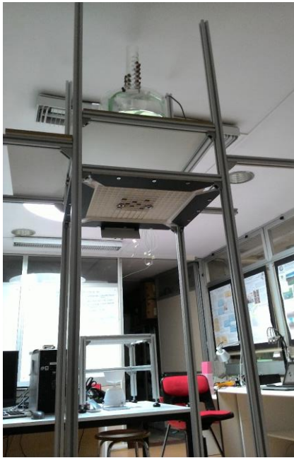
Figure 1: Picture (a) and schematics (b) of the rain simulator developed at the University of Genova for testing non-catching type gauges.
