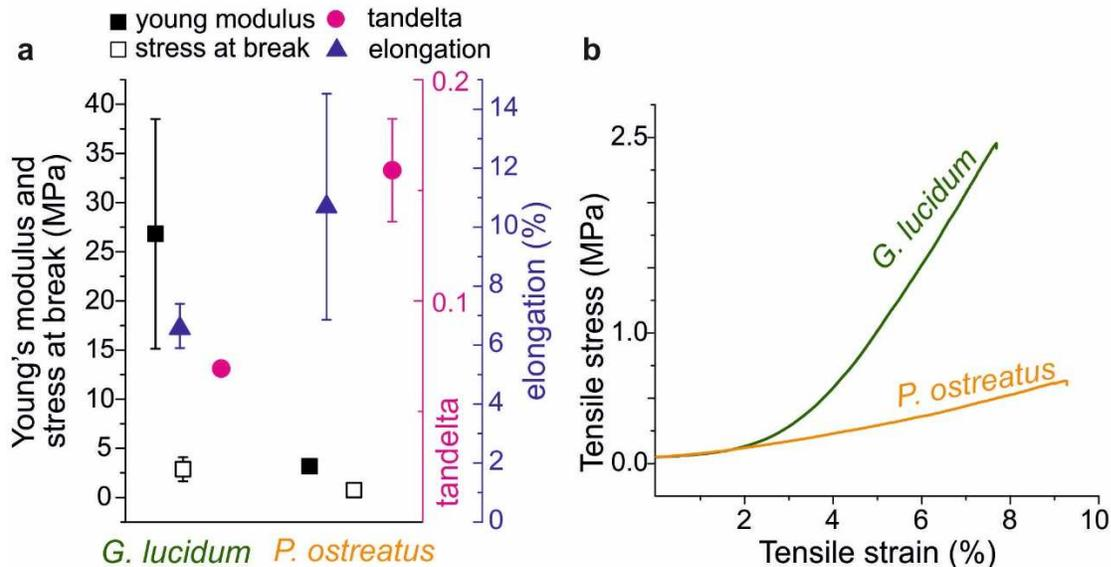
**Figure 1.4.** Mechanical features of mycelia. (a) Young modulus, stress at break and elongation results after the tensile test; tan $\delta$  values after DMA analysis. (b) Tensile test curves of the two mycelia under study.
