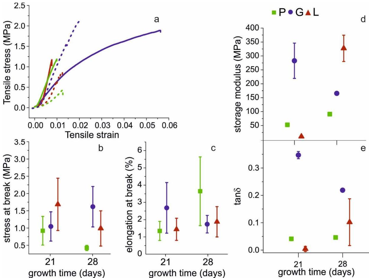
**Figure 1.7.** Mechanical properties. a) Stress strains curves of different samples collected after 21 (straight lines) and 28 days (dotted lines), analyzed by tensile test. b,c) Average stress and elongation at break of different samples collected after 21 and 28 days, from tensile test curves. d,e) Storage modulus and  $\tan\delta$  calculated by DMA on mycelia collected after 21 or 28 days of growth.
