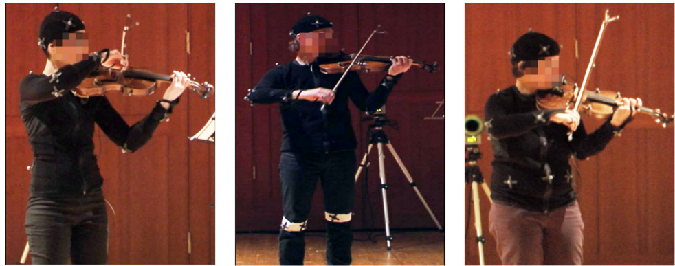
Fig. 1 The violinist MOCAP setup: markers are placed over subject, bow, and violin
