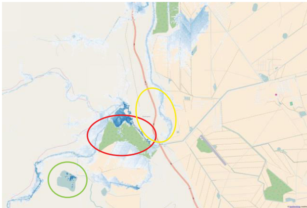
Figure 9 Effect of forest (red circle) and built-up areas (yellow circle). An open water body (indicated by a green circle) gives a noisy signal.
