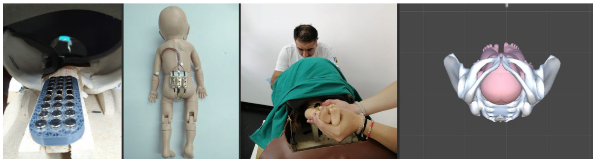
FIGURE 7. (a) The magnetic matrix is installed inside the birth simulator eBSim, 205 mm above the ischial spines, covered by a 1 mm soft layer (not shown). (b) Hall-effect sensors used to detect the engagement level of the head. Such sensors are located on the fetus, 205 mm from the biggest diameter of the head. (c) The head is positioned on in the birth canal so that midwives' students can assess the engagement level which is also measured by the magnetic transducer. (d) The fetal position is displayed in real time in a virtual representation.
